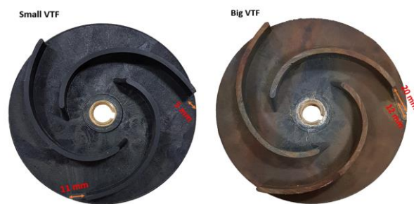
Figure 3. Vane tip fault.
