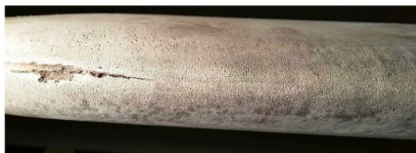
Figure 2. Example of a blade damaged by a longitudinal crack [4]
